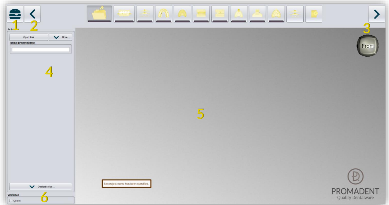
image 2: The BiSS program after launch 1) Menu: Contains settings, about us, other applications, new project. 2) Back: get back to the step before. 3) Next step: Complete the current processing step and proceed to the next step. 4) Action window: Individual for the respective work step. Here: Load file and define the work steps. 5) Work surface. 6) Visibility switch: Visible after loading the scans.
