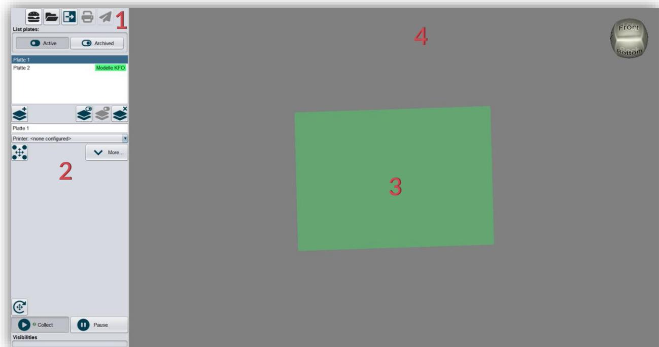
*image 2: The BiSS program after the start. 1) Menu: Contains settings, printer configuration, about BiSS. 2) Action window: Individual for the respective work step. 3) Work area/printer plate. 4) Plate activities.*
