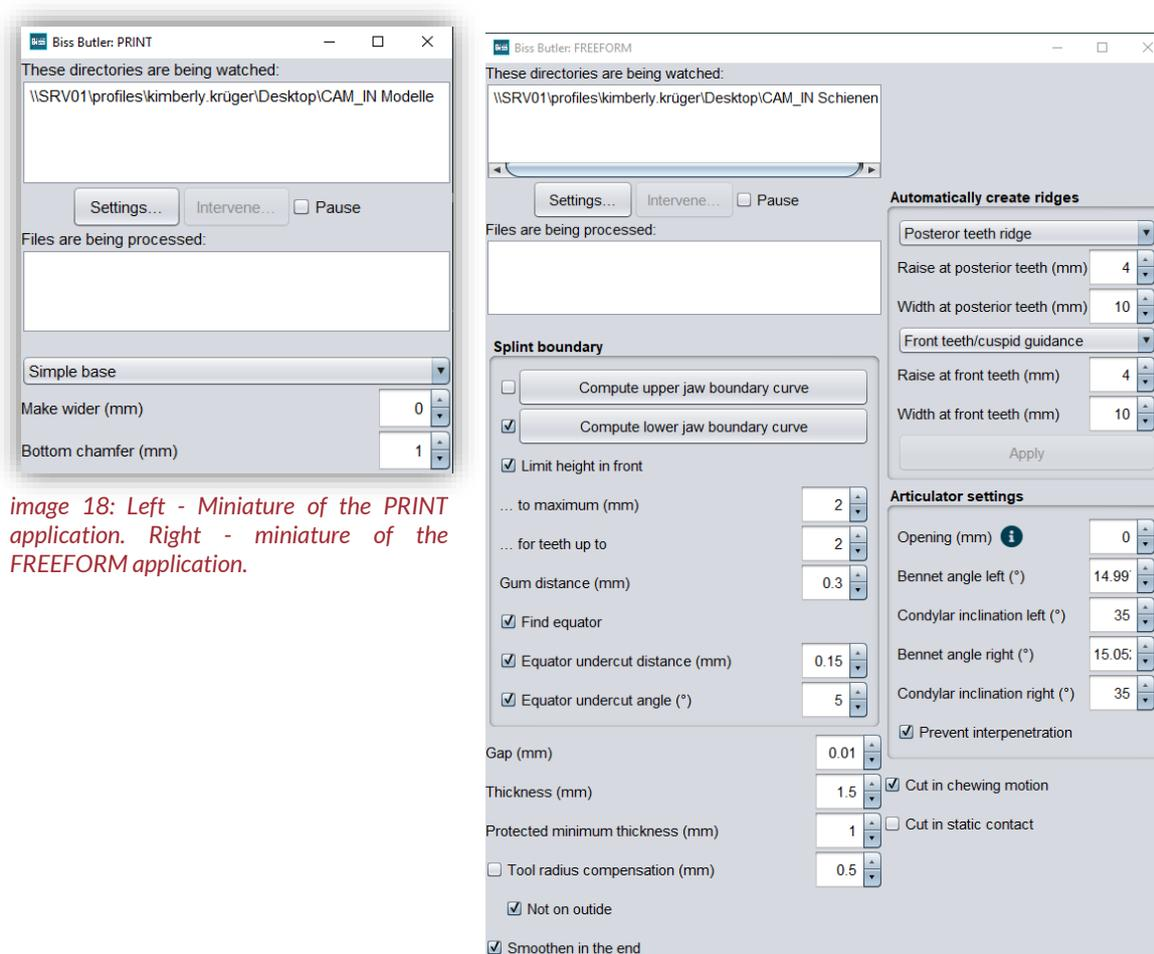
image 18: Left - Miniature of the PRINT application. Right - miniature of the FREEFORM application.
