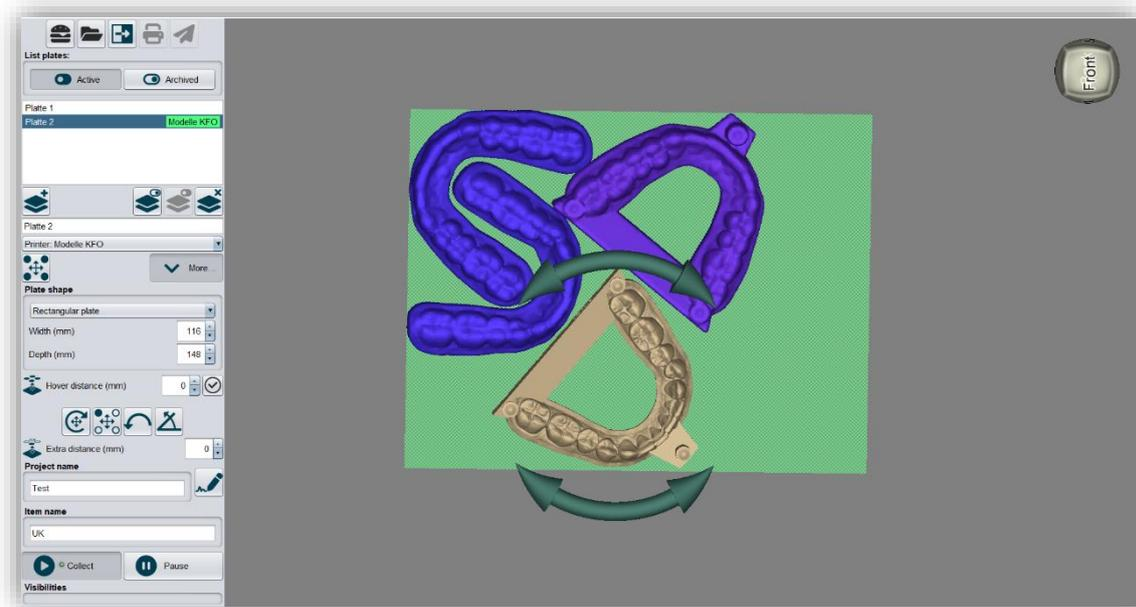
*image 16: View of the loaded meshes on the printer platform.*
