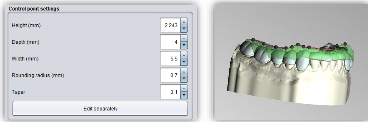
image 37: LEFT: Selection options for ridges in the anterior region RIGHT: View after selecting a control point
